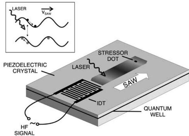
Schematic sketch of a SAW sample for the acoustically driven transport of electron hole pairs. The material of the system may be, for example, GaAs for the piezoelectric crystal, InGaAs for the quantum well, and InP for the stressor. The inset depicts the storage of optically generated excitons in the potential of the surface acoustic wave. These spatially separated excitons may recombine at the location of the quantum dot, given rise for the generation of single photons.
