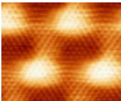
Atomically resolved image of the graphene overlayer. The image shows three different levels of apparent heights, namely four bright maxima, a dark minimum in the center between the three maxima on the right hand side, and a less dark minimum between the three maxima on the left hand side.  $50 \text{ \AA} \times 40 \text{ \AA}$ ,  $I_t = 1 \text{ nA}$ ,  $V_{\text{sample}} = -0.05 \text{ V}$ .
