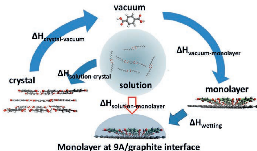
Scheme of the proposed Born-Haber cycle. \Delta H_{\text{sol-monolayer}} (red arrow) is not directly accessible, but a detour via crystal, vacuum, and unsolvated monolayer (blue arrows) as defined reference states facilitates quantification of the overall enthalpy difference.
