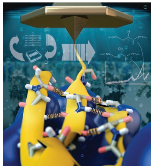
Fig. 1: The combination of steered molecular dynamics simulations (SMD) and AFM single-molecule force spectroscopy (cantilever shown in gold) allows testing and fine-tuning the mechanical stability of cellulosomal scaffoldin protein domains (secondary structure of the molecule represented in yellow, hydrogen bonds represented by springs). One mutation, predicted by SMD, doubled the mechanostability (grey schematics) [3] .
