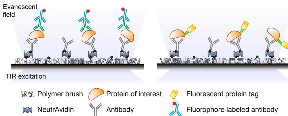
Figure 1: Schematic for single molecule immunoprecipitation.
