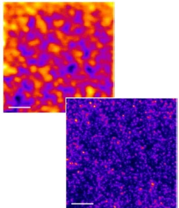
Fig. 2: Conventional confocal image of 20 nm fluorescent beads limited by the diffraction limit of light (upper left side) and corresponding super-resolved STED image of the same area (lower right side). Scale bars 1  $\mu\text{m}$ .
