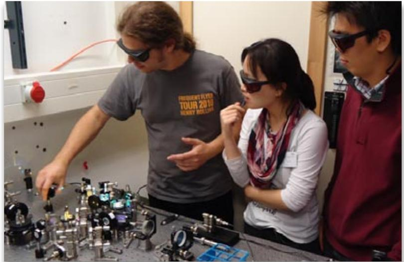
This module took the students through each step of aligning a self-built STED microscope. First it was shown how to select a certain wavelength range for the depletion beam using a prism-based monochromator and its importance for the success of the experiment was discussed. Furthermore the adjustment of the donut beam and its crucial contribution to the setup was explained and performed by using specialized components to analyze its circular polarization.
