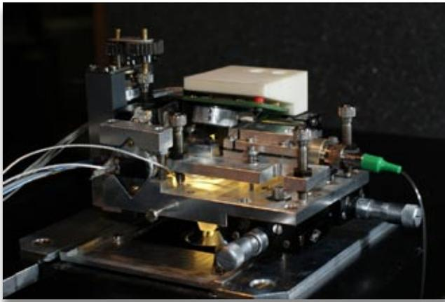
Figure 1: Experimental setup. The force-extension traces were recorded with a custom built AFM head specialized for long term SMFS data acquisition.
