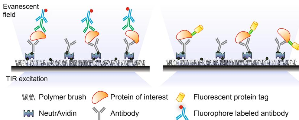
Figure 1: Schematic for single molecule immunoprecipitation.
