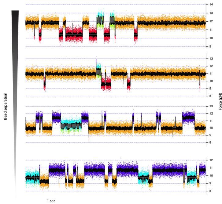
Figure 3: Rapid transitions between several states can be observed. By changing the trap center positions different pretensions can be applied to the protein, thus shifting the equilibrium between the states.
