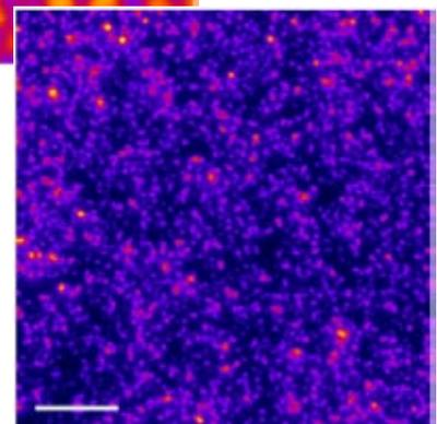
Fig. 2: Conventional confocal image of 20 nm fluorescent beads limited by the diffraction limit of light (upper left side) and corresponding super-resolved STED image of the same area (lower right side). Scale bars 1  $\mu\text{m}$ .
