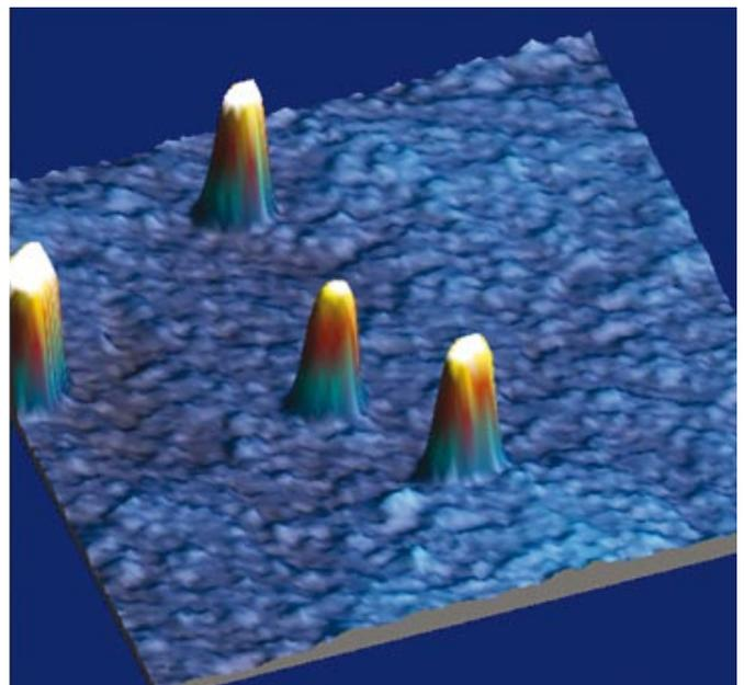
*Atomic force microscope image taken of an InAs quantum dot sample. The dots are approximately 10nm high.*
