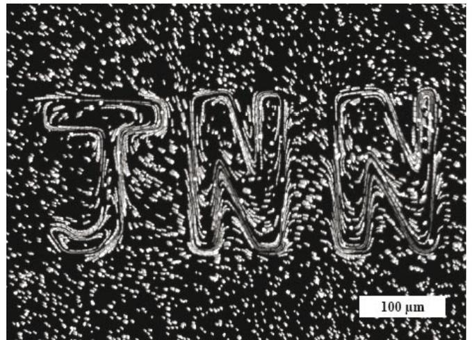
*Pumping water optically without walls along a freely defined pattern. Fluid flow is driven by a laser scanning microscope. Complex flow patterns are easily accomplished. Pumping is a result of small fluid movements for each passage of the laser focus. Water flow is visualized by overlaying the difference of successive pictures.*
