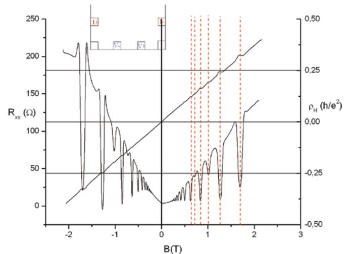
Sample resistance versus magnetic field. Measurements are performed at ultralow temperatures (300mK).
