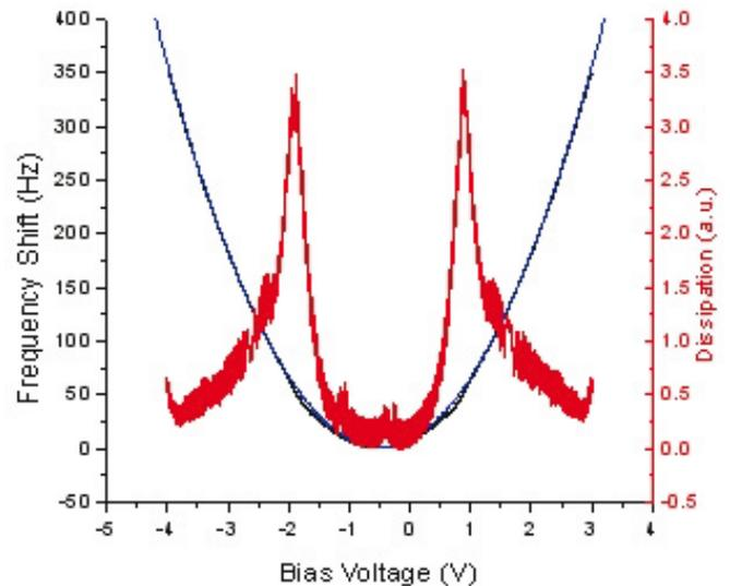
*Response of the cantilever to a voltage sweep while positioned over a quantum dot. The electrostatic force is quadratically dependent on the voltage, which is apparent in the frequency shift of the cantilever (black). The blue curve is a parabolic fit. The dissipation (red) refers to the energy required by the cantilever to maintain its oscillation amplitude.*
