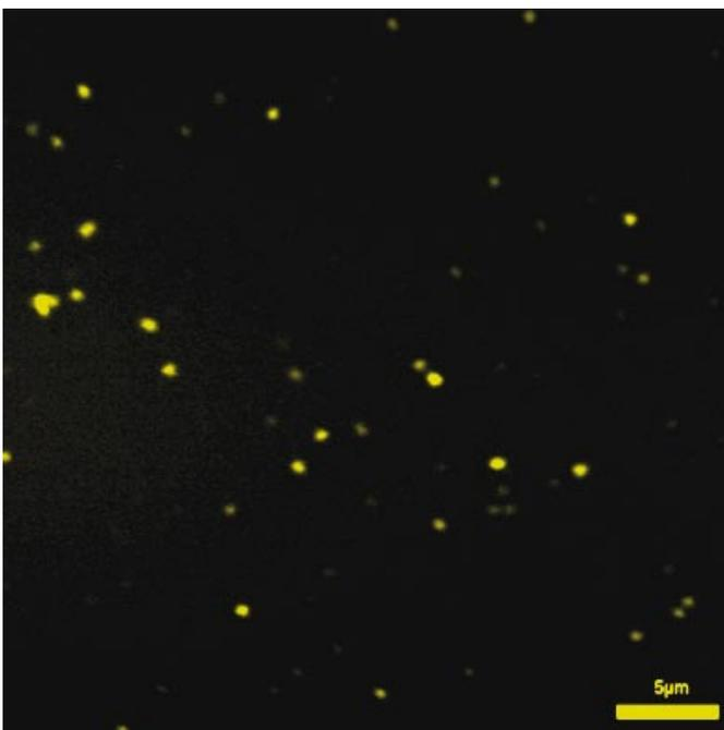
THG image of 40nm gold nanoparticles. Excitation wavelength  $\lambda = 1200\text{nm}$  and emission filter 400/20.
