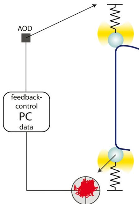
*Scheme of the experimental setup. An actin filament (blue) is suspended between two beads held in the optical traps (yellow gradient and springs). The lower bead's image on a photo quadrant diode gives information about the applied tension that is used in a PC-controlled feedback-loop to adjust the position of the upper bead via an acousto-optical deflector (AOD).*
