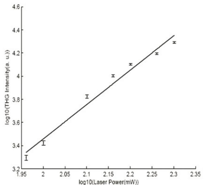
THG signal (log. scale) versus laser power (log. scale). A linear regression best fit yields a slope of  $3.0 \pm 0.4$ .
