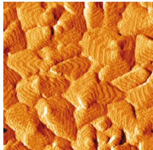
AFM picture (size:  $2 \times 2 \mu\text{m}$ ) of a 12nm thick pentacene-layer on  $\text{SiO}_2$ .
