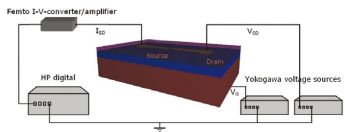
Setup for electronic characterization.
