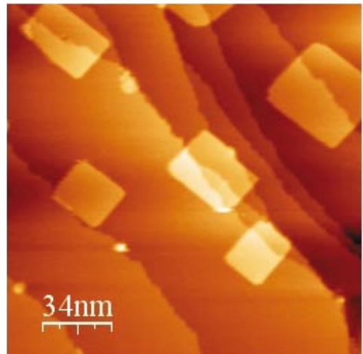
NC-AFM topography image showing first and second monolayer coverage of KBr on Cu(100).
