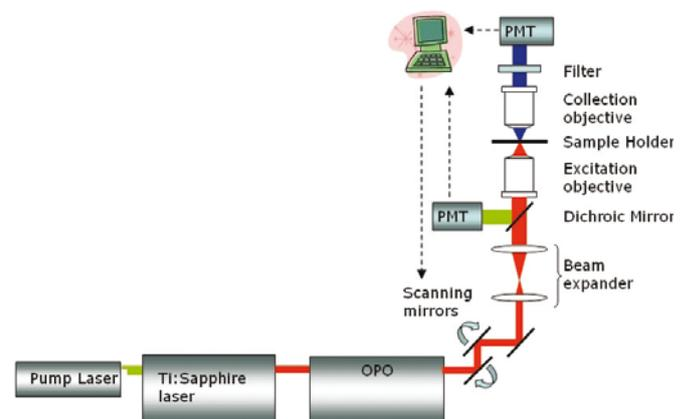
Schematic of THG/MPF microscope.
