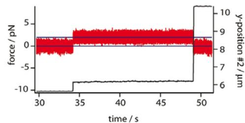
*Example trace. When the feedback is started, the position of the upper bead (black) is changed to apply a constant tension of  $\approx 2\text{pN}$  (red). When the filament ruptures, the upper bead jumps to a maximum position.*
