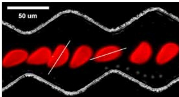
Fig. 1: Orientational oscillation of a vesicle in a wide structured channel. The image is a superposition of video frames taken at time intervals of 1 s. The tilt angle oscillates as indicated and is a measure of elastic properties.
