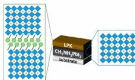
Schematic representation of a hybrid perovskite film composed of a MAPI/LPK bilayer.
