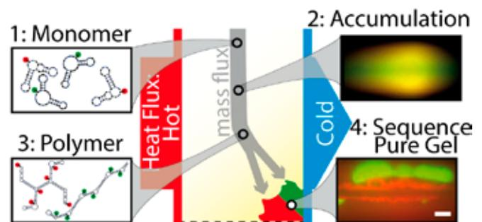
DNA strands that can fold into multiple hairpins are selected against their imperfect siblings with single base mutations by their gelation in a thermal trap. Slight sequence differences within the gel-forming strands lead to their separation into spatially distinct, sequence pure oligomer gels.
