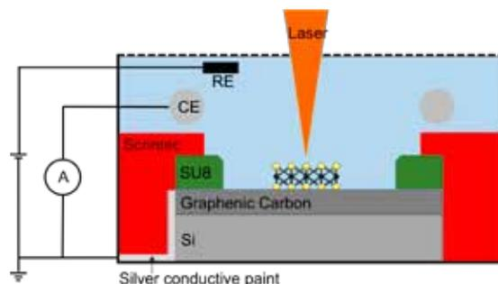
Electrochemical cell consisting of a graphenic carbon substrate covered with an electrically insulating photoresist (SU8). A 100 μm diameter window enables the contact between electrode and electrolyte and the positioning of single MoS<sub>2</sub> flakes with known geometry.
