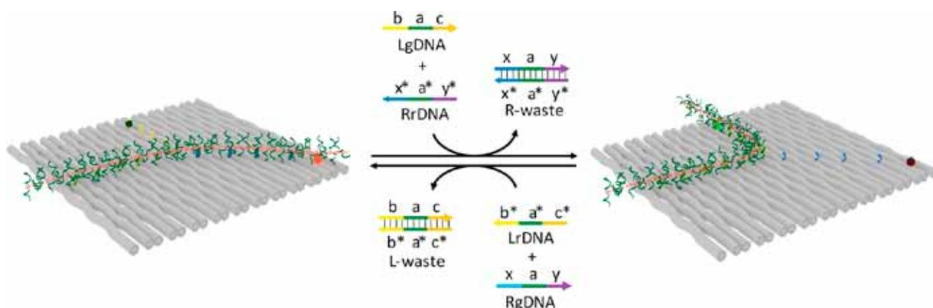
Figure 1. Illustration shifting the position of a poly(DNA-phenylene vinylene) on DNA origami.<sup>4</sup>
